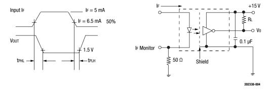
Figure 4. OLI600 Switching Test Circuit
