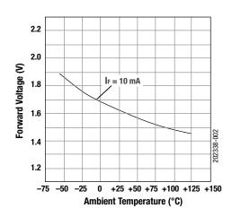
Figure 2. Forward Voltage vs Temperature
