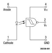
Figure 1. OLI600 Block Diagram
