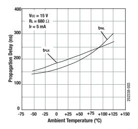
Figure 3. Propagation Delay vs Temperature
